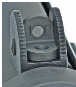
The Sterling L2A3's flip rear peep sight has apertures for 100 and 200 meters, while the blade front sight can be turned in or out to regulate elevation zero.
