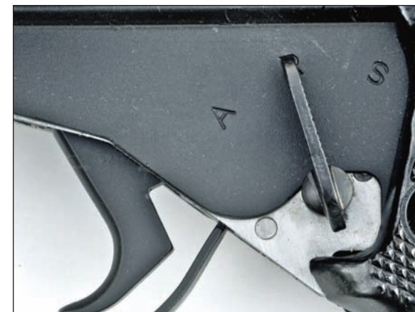
The three selector positions on the CPS L2A3 are marked "S" for safe, "R" for the British term "Repetition" or semiautomatic fire and "A" for full-auto.
